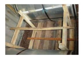
The space between two steel coils, use one wooden structure/timberwork to secure and sustain the gap. 相邻两卷间的空档用 2 组木架支撑,之间用木条连接
