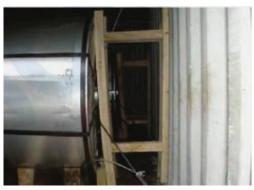
Left/Right side, use two wooden structures /timberworks to secure and sustain each coil 每个卷左右两侧各用 2 组木架支撑固定
